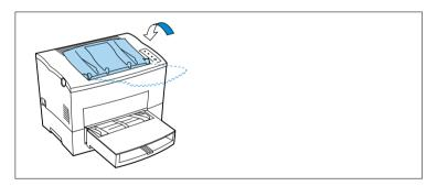
3 Press the top cover release button and open the cover.
